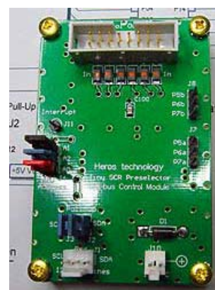
I2C bus control module.
