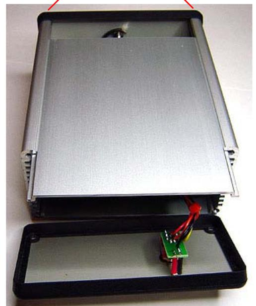
Remove the lid from the local oscillator section.
